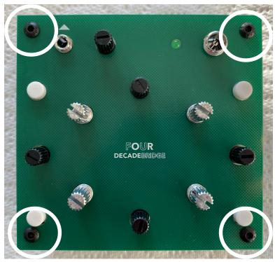
Turn Four over and make sure that the LED has dropped into the hole on the faceplate. Solder all the parts into place before cutting the excess off the LED legs.
