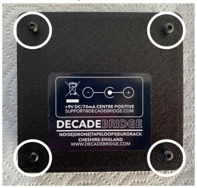
Now you can insert Four into the case. Holding it firmly in place, continue to screw the hex screws so that they feed into the standoffs. If they do not take, back them off slightly and slowly try them again. You may need to screw each one in gradually to start with before going around and tightening them all up.
