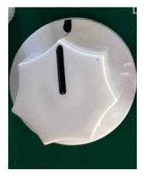
Set the trimmer pots so that the gap in each pot is vertical. This is the midway point. Push the smaller white knobs on to the pots so that the markers are pointing directly up.
