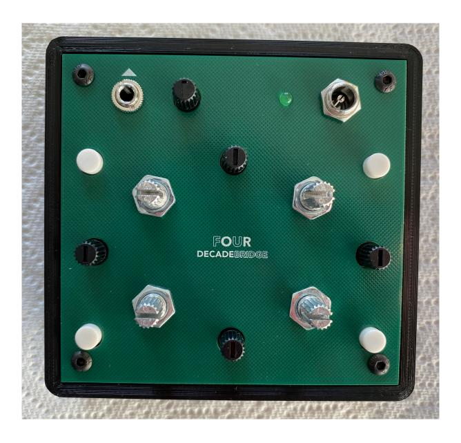
The last thing to do is add the knobs. Set the 4 pitch potentiometers so that the gap in the shaft is horizontal. This is the midway point of the turn. Place the large white knobs so that the markers are pointing directly up.
