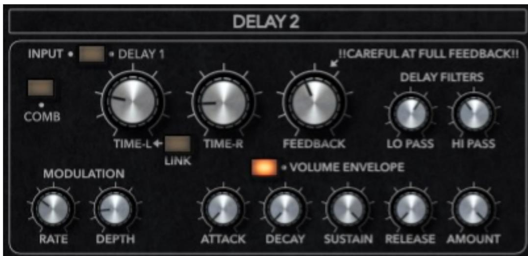
Both delays have 2 different time settings, **'COMB'** (comb filter) or **'DELAY'**. The time of the delay can be set for both the left and right channels with **'TIME-L'** and **'TIME-R'**. **'TIME-R'** can also be linked to **'TIME-L'** using the button **'LINK'**. Below the time knobs is the delay's **'MODULATION'** section. The **'RATE'** and **'DEPTH'** of the modulation is set here.
